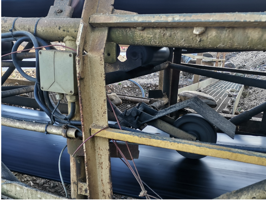
Figure 1.1: A conventional electronic belt scale.
