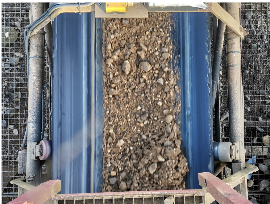
Figure 4.4: The view of the conveyor belt and material as seen by the sensor.
